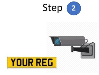
Camera, using ANPR, checks database to see if vehicle is eligible to enter or not (has a permit)
